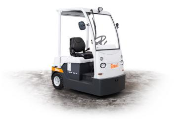
3-wheel tow tractor, with on-board operator and rear-wheel drive. Extremely compact and easy to drive, ideal for all industrial duties - both indoors and outdoors.
